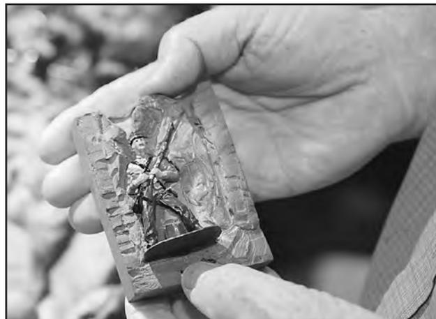
Making soldiers involves creating a mold out of an original figure from epoxy and hardener. The mold is split in half and rejoined, then molten pewter, at about 600°F is poured into the mold. After about ten minutes, the mold is pulled apart and later Ron paints the details, even the lips on the faces, using very fine brushes and enamel paint (see photo below).
